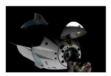
The Dragon's docking showcased one of the biggest features of SpaceX's capsule: its automated docking system. The vehicle is designed to autonomously approach the ISS and latch on to a standardized docking port, without any input from its human passengers.
